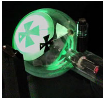
Figure 1 – An illuminated Crookes Tube. The metal 'Maltese Cross' in the centre of the tube is casting a shadow on the anode at the rear of the tube. ( http://www-outreach.phy.cam.ac.uk/camphy/electron/electron1_1.htm )
